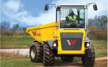
Wheeled Dumpers - Traditional and Dual View Articulated wheel dumpers are excellent for moving bulk materials. With our Dual View dumpers, the operator can quickly and comfortably change the seat and console position to keep the task front and center. The entire operating platform rotates 180 degrees, giving the best view while working or driving the machine.
